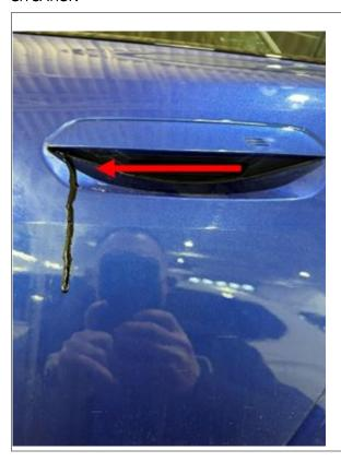
Black resin is leaking from below the outside door handle(s).
