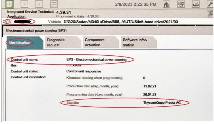
2. On vehicles with the TKPS EPS, replace one or both tie rod assemblies as per REP 32 21 231.
