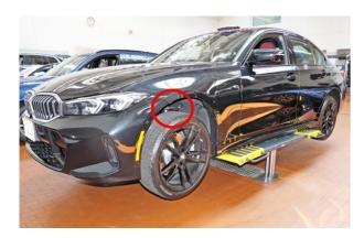
The left front suspension's aluminum strut dome (general area circled) was incorrectly riveted to the body's wheel-well. Overtime, corrosion can form around the rivet holes. Structural integrity would thereby NOT be reduced, because the primary strength of that dome attachment is from structural adhesive.
