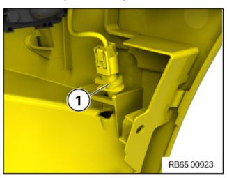
• Unclip temperature sensor (1) from the front bumper panel to the top.
