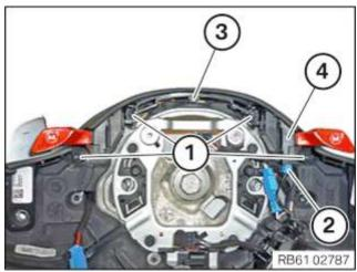
Installing the cover for the M Sport steering wheel
