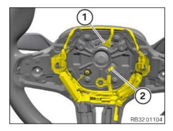
• Connect and lock the connector (1) and (2).
