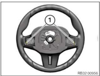
• Unlock plug connection (1) and disconnect.
