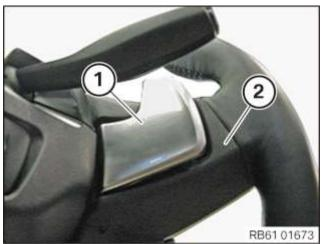
• Insert the access line (1) into the rear of the steering wheel (2).
