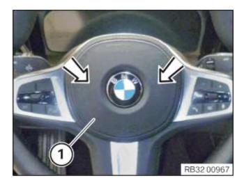
• Press the airbag unit (1) with even pressure in the arrow direction into the steering wheel.
