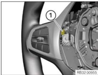
• Tighten screws (1) on the back of the steering wheel.
