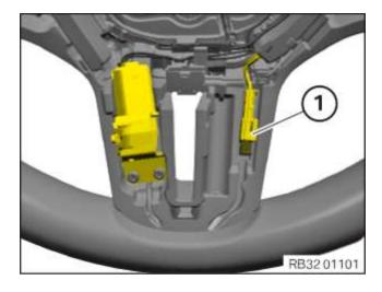
• Unlock plug connection (1) and disconnect.
