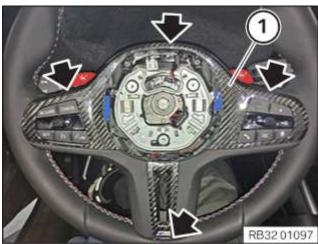
Check the detents (1) for damage.
