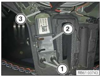
Removing the impact plate (M Sport steering wheel)
