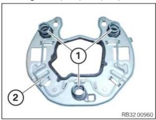
• Check the position of the springs (1) on the impact plate (2), correct if applicable.
