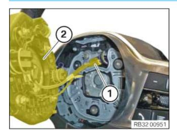
• Connect and lock the connector (1) of the airbag unit (2).
