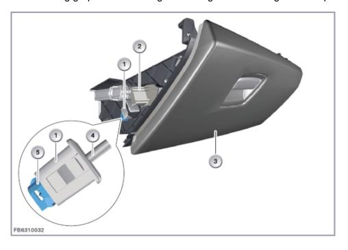
tcn is activated mechanically. A stop element presses against the switch pin when the glove box cover is. This interrupts the circuit. The stop element is connected to the glove box cover.
