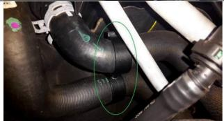
Close up view of spacer installed.
