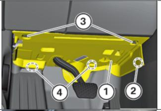
If the complaint still occurs after installing the spacer, the following must also be done: Remove the trim panel for pedal mechanism. See repair instructions REP 5145186
