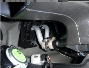
Tape the two heat exchanger lines with a felt strip (part number: 51 45 2 353 024) 4-5 inches (10-12 cm) long around each of the lines. Secure the lines together using a worm-type hose clamp (part number 07 12 9 952 117). This prevents the lines moving in the aperture grommet.
