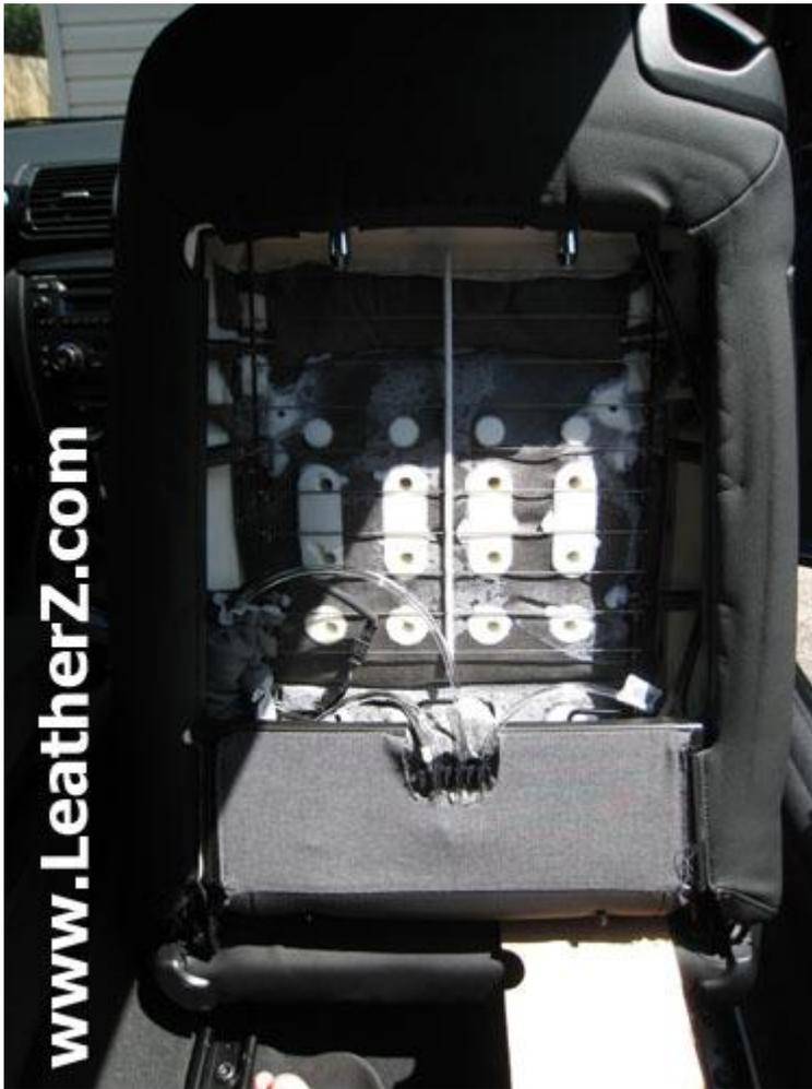
With the setback removed, you can remove the remnants of the clips. The clips are a bit tough, they push in easy but do not pull out easy. I was able to reach down (thin, long hands) into the seat and feel the other end of the clips. Then I just pushed the clip up into the seat and removed it from the top. You will want to make sure your hands can fit in this way before pushing the clips up as you may not be able to get the clips out.
