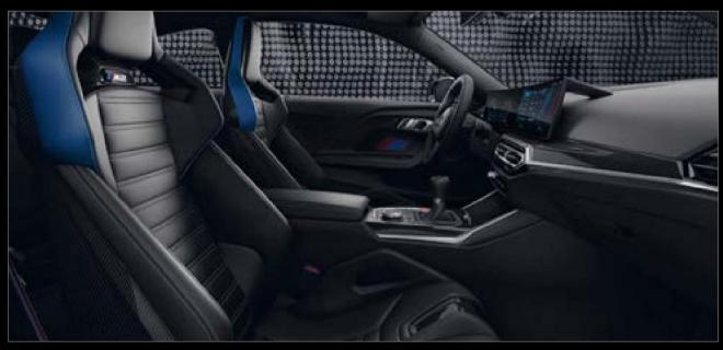
ÿ The M carbon bucket seats1,2 with illuminated model lettering and visible carbon surfaces ensure weight reduction in the vehicle. They can be electrically adjusted in many ways and are suitable for multi-point seat belts.
