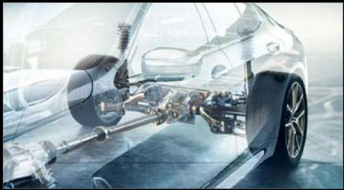
ÿ The M Sport differential optimizes traction and driving stability when changing lanes and accelerating out of bends, at high cornering speeds and on different road surfaces. The traction is optimized via an electronically controlled multi-disc lock to reduce the speed differences between the rear wheels.
