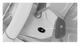
Drive-ready state cannot be switched on if the vehicle key is not detected.
