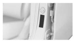
The tyre inflation pressure information is located on the body pillar of the driver's door.
