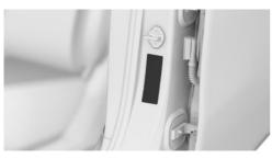
The tyre inflation pressure information can be found on the tyre pressure label on the body pillar of the driver's door.
