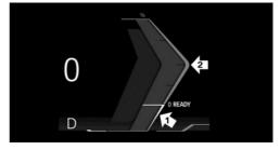
Needle in the arrow 1 area: display of the energy recuperation achieved, for example during deceleration. CHARGE.
