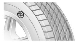
The icon identifying run-flat tyres is a circle with the letters RSC on the tyre sidewall.
