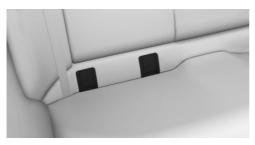
The fixtures for the lower anchors are located behind the marked covers. To expose the anchorage points, open the flaps upwards.
