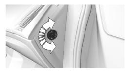
The key switch for front passenger airbag is located on the outside of the dashboard.
