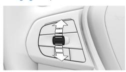
Press the rocker switch repeatedly up or down until the desired speed limit is set.
