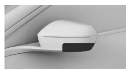
An exterior mirror camera is located under each exterior mirror housing.
