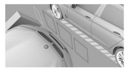
Obstacle markings are displayed at the sides of the vehicle to protect the vehicle's flanks.
