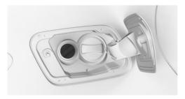
The fuel filler cap for the reducing agent is located next to the fuel filler cap for the fuel tank.
