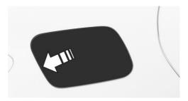
2. Turn the fuel filler cap anticlockwise.
