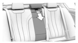
Pull the lever and fold the centre section forwards.
