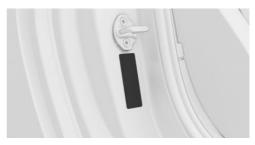
The vehicle identification number is on the type plate on the right-hand side of vehicle.
