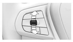
While the system is interrupted, press the rocker switch up or down once. The system is activated.
