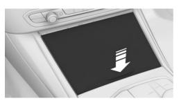
2. The socket is located between the cup holders. Pull off the cover.
