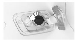
3. Place the fuel filler cap in the holder on the fuel filler flap.
