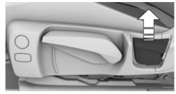
Pull the lever and add or remove pressure on the backrest as required.
