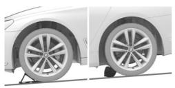
If it is necessary to change a wheel on a slight downhill gradient, place chocks and other suitable objects, for example stones, under the wheels of the front and rear axles against the direction of roll.
