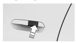
Hold the NFC antenna on the smartphone directly and centrally up against the outside door
