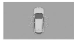
The maximum door opening angles are displayed when the selector lever is in position P.
