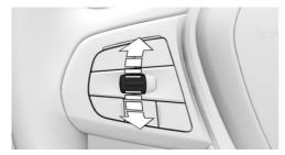
Press the rocker switch repeatedly up or down until the set speed is set.
