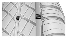
There are wear indicators from the tyre manufacturer distributed over the tyre circumference with a height of at least 1.6 mm, approx. 0.06
