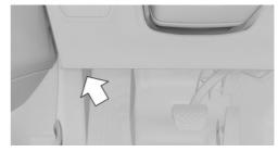
There is an on-board diagnostic socket on the driver's side for reading out vehicle data.
