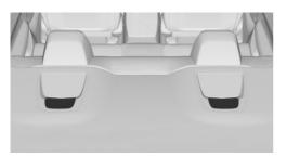
There are two attachment points for the upper retaining strap of ISOFIX child restraint systems.
