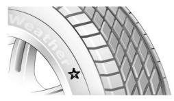
Certain makes of tyre are recommended by the manufacturer of the vehicle for each tyre size. The tyre brands can be identified by a star on the tyre sidewall.
