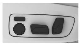
The switches for the seat settings are located at the front seats.
