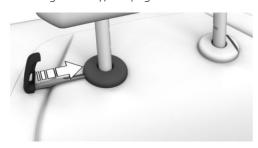
4. Press and hold the integrated key and the button simultaneously, arrows 1, and pull the head restraint fully out.
