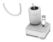
Let the compressor run for max. 10 minutes to fill in the tyre sealant and reach a tyre inflation pressure of 2 bar.
