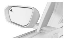
The light in the exterior mirror flashes if other vehicles are detected by the rear sensors when the vehicle is reversing.
