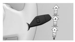
To activate: press the lever upwards once from position 0, arrow 1.
