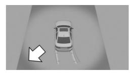
In the Park Distance Control view, the relevant boundary area flashes red if the sensors detect vehicles.
