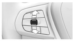
Press the rocker switch repeatedly up or down until the set speed is set.
