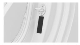
The vehicle identification number is on the type plate on the left-hand side of vehicle.
