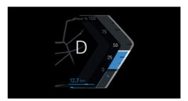
When driving efficiently, the power display is coloured blue.
