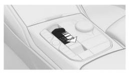
Pull the selector lever out of selector lever position D to D/S.
